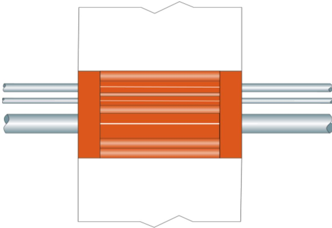
Figure 12. Principle of NOFIRNO sealing system with cable penetrations in vertical walls with thickness of minimum 100 mm up to 260 mm. The penetrations shall be completely filled.
