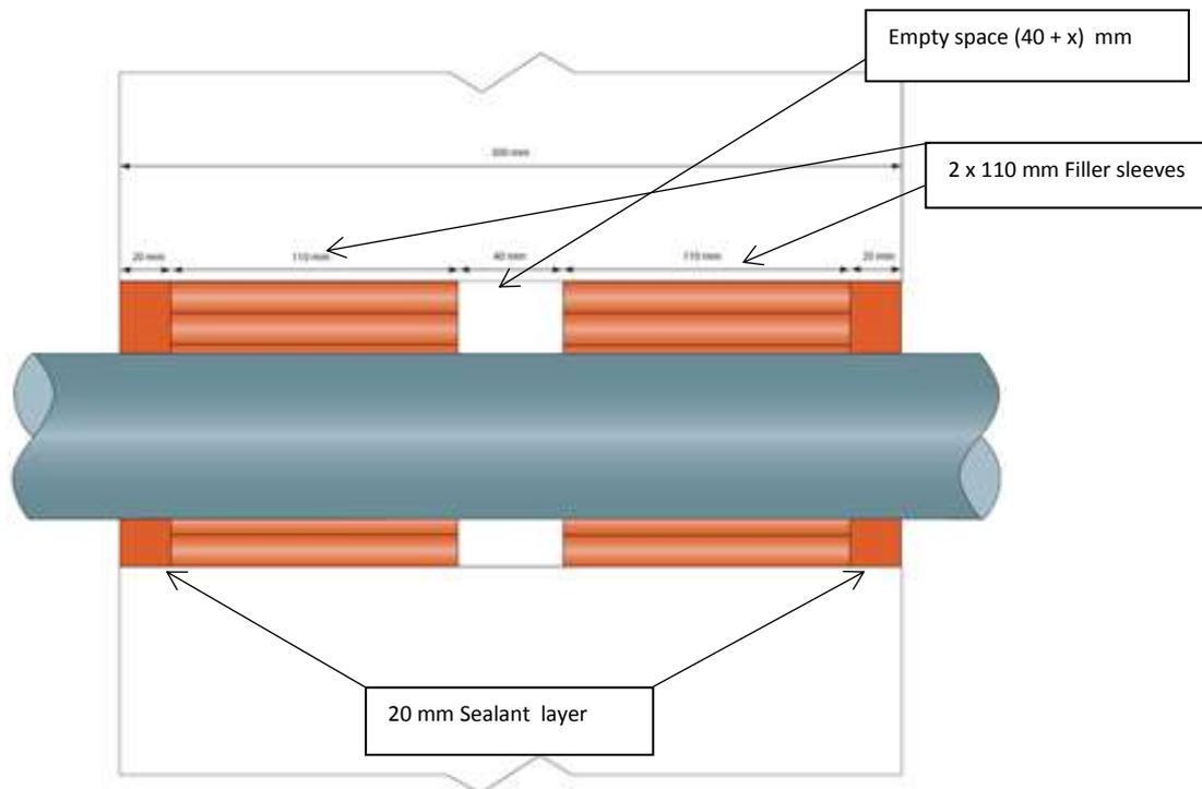
Figure 7: Principle of NOFIRNO sealing system with single pipe penetration in (300 + x) mm wall
