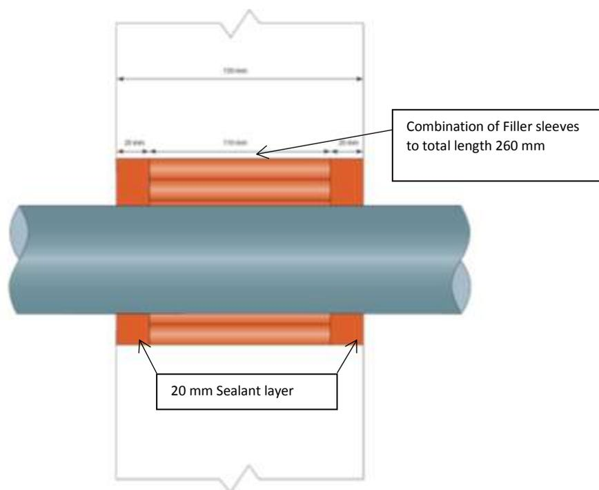
Figure 8: Principle of NOFIRNO sealing system with single pipe penetration in 300 mm wall
