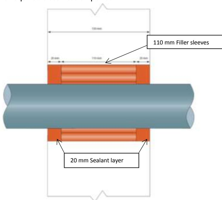
Figure 6: Principle of NOFIRNO sealing system with single pipe penetration in 150 mm wall or floor
