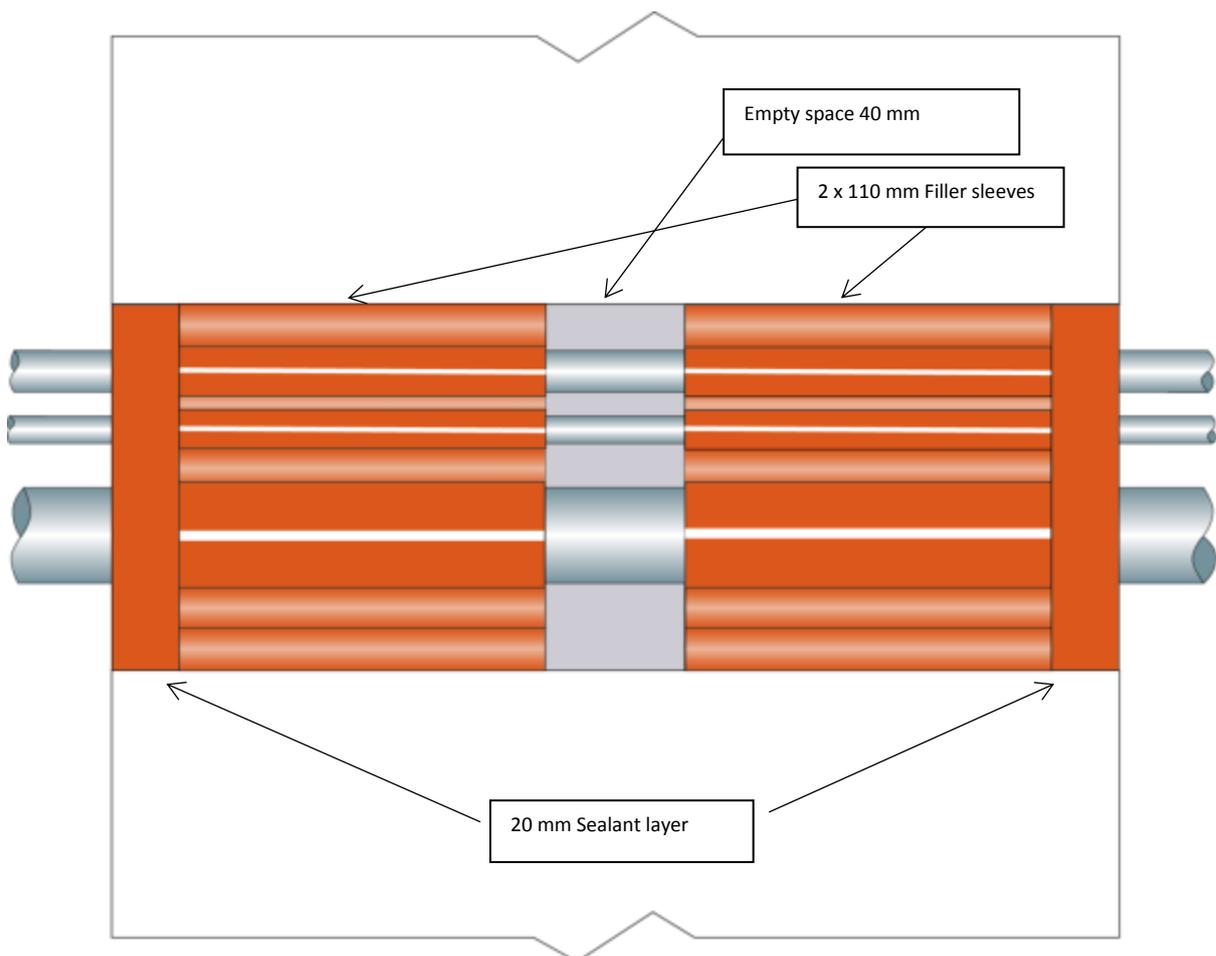
Figure 13. Principle of NOFIRNO sealing system with cable penetrations in vertical walls with thickness of minimum 260 mm. In the centre of the penetration an empty space may be present. The figure shows as an example a cable penetration in a 300 mm wall.
